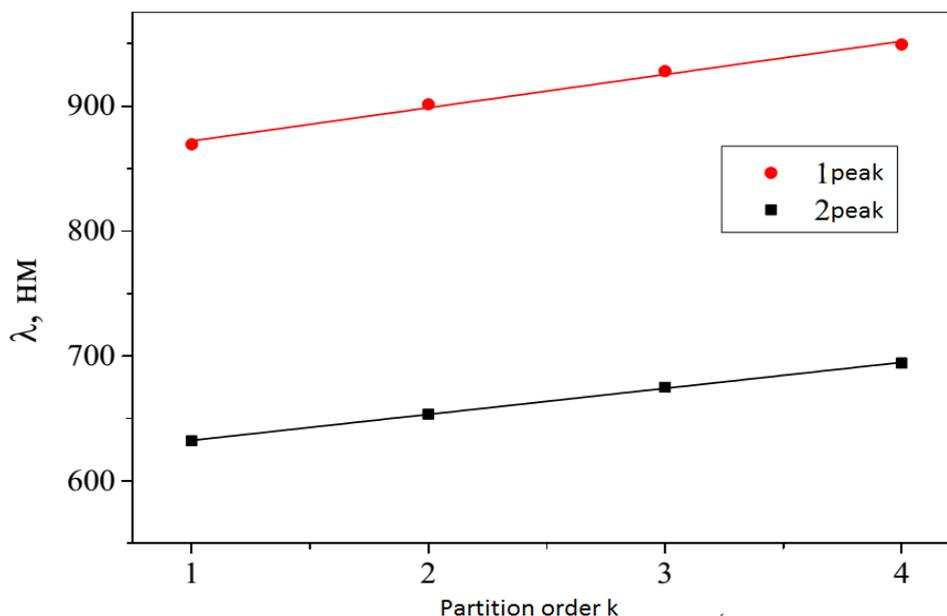
Fig.5. Dependence of the peak positions of the minima of the negative refractive index of the order of partition  $k \Omega k$  structure with period  $d = 300$  nm
