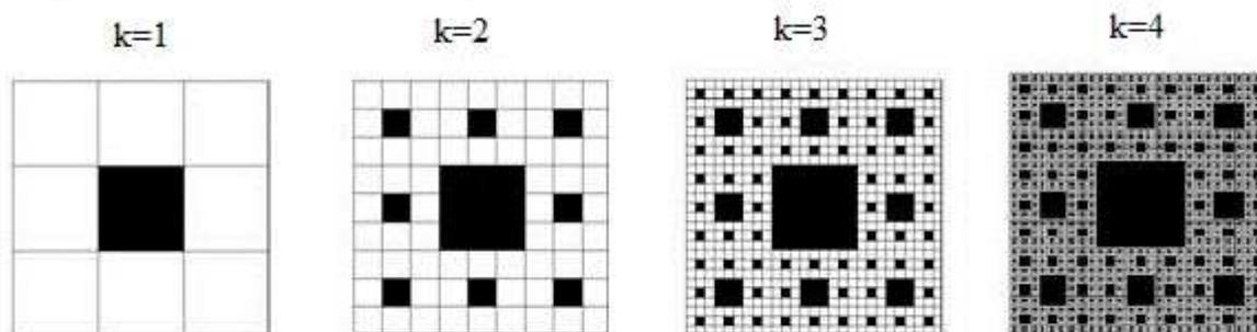
Fig.1. Structure of the unit cell of traditional and fractal mesh metamaterial at different orders of partition  $k$
