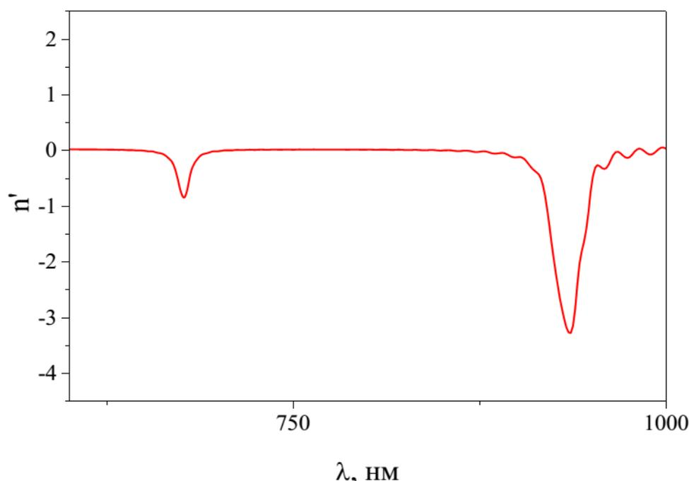
Fig.4. Spectral dependence of the real part of the refractive index for the structure with a period of  $d = 300$  nm and the order fractal partition  $k = 3$
