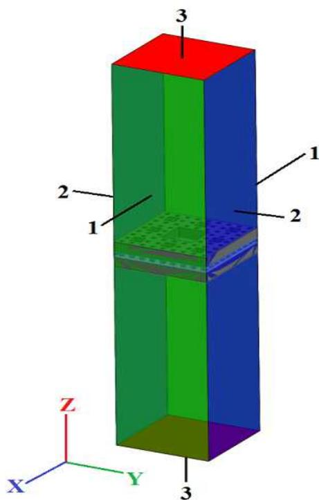
Fig. 3. The boundary conditions on the edges of the modeling area: 1 – an ideal electrical conductor, 2 – an ideal magnetic conductor, 3 – an open border; a waveguide port
