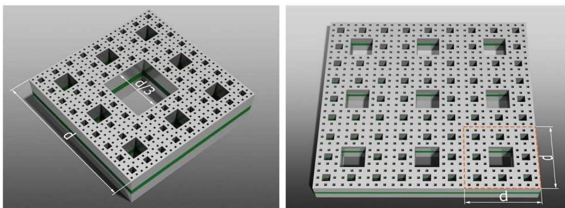
Fig.2. Single cell mesh fractal metamaterial ( $k = 4$ ) and a fragment of the structure of the metamaterial with a period  $d$  ( $k = 3$ )
